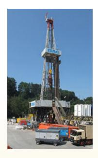
Derrick at St. Gallen geothermal project. Courtesy Creative Commons by Kecko; Licensed under CC BY 2.0. Geothermal drilling rigs are indistinguishable from oil and gas rigs. St. Gallen in Switzerland was temporarily sealed in 2013 after a gas kick and earthquake, and is now used for research.
