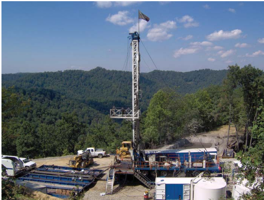
EQT drills into the Lower Huron shale at this eastern Kentucky well site.
