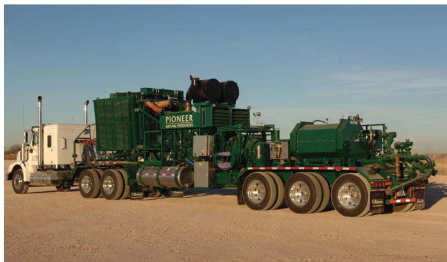
A new hydraulic frac truck in the Eagle Ford shale is among a fleet owned by Pioneer Natural Resources Co. Pioneer and others are acquiring their own frac fleets to cut “cost creep” for outside services and to assure availability which is tight.
