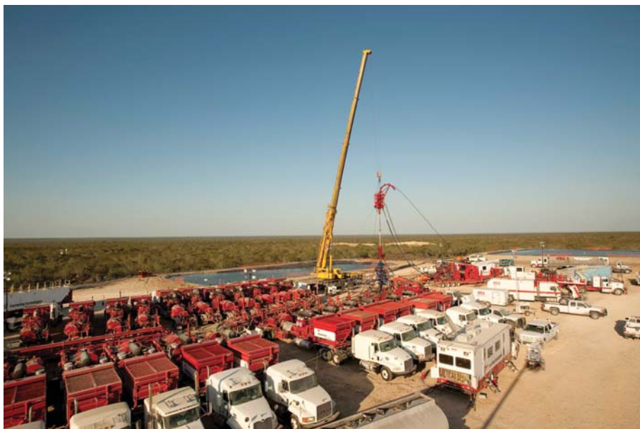
A hydraulic fracturing fleet in the Eagle Ford shale is on site for a 17-stage completion of a Swift Energy Co. well with a 6,000-ft horizontal leg. Multi-stage frac techniques are boosting recoveries from the shale play.
