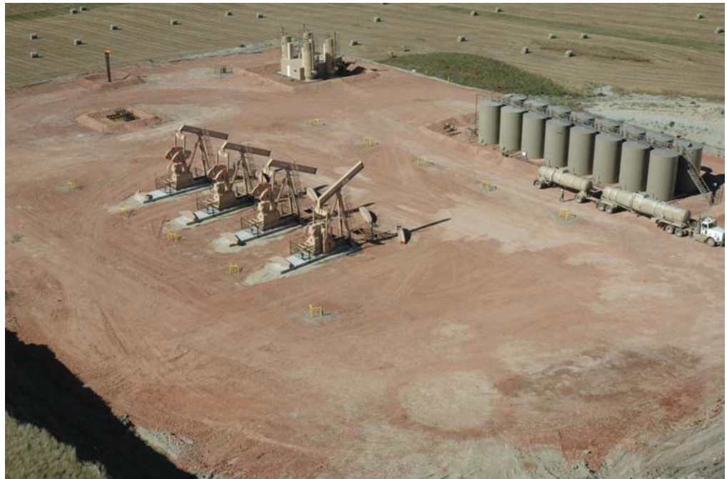
Continental Resources Inc. drilled these four wells in the greater Bakken from a single pad with an 800,000-pound rig that walks on hydraulic feet between drill sites. That eliminates dismantling time. The single pad and walking rig have reduced costs.
