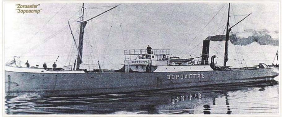
The first-ever oil-carrying steam ship, Zoroaster, commissioned by Ludwig Nobel and built in 1877. Photo courtesy of the Azerbaijan National Archives and Petroleum History Institute.
