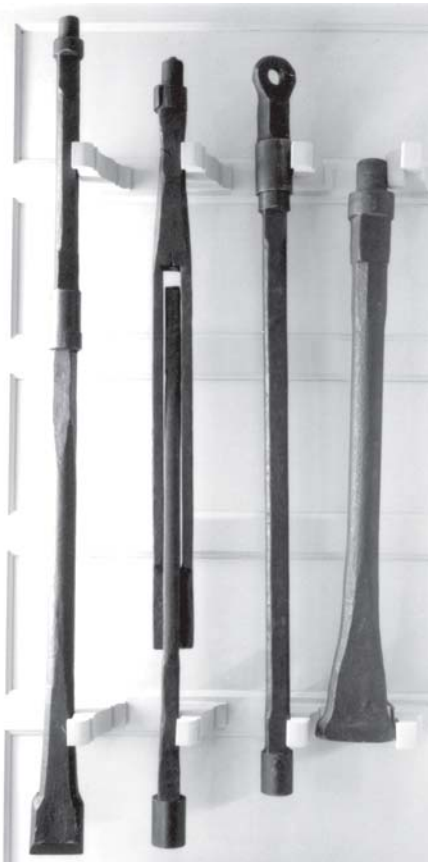
Tools made by William Smith to drill the Drake well. Courtesy Drake Well Museum Archive-Pennsylvania Historical and Museum Commission.
