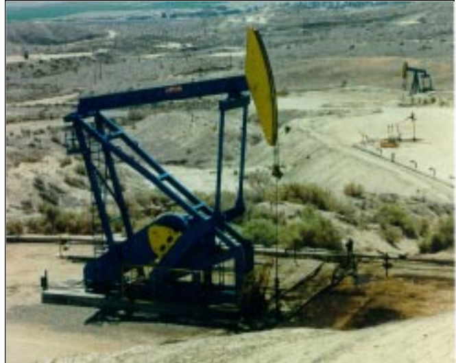
This beam pump, used to reduce back pressure in a well and increase production, is one of many artificial-lift units in the Elk Hills field. To analyze the production history, Ryder Scott had to consider the extent of artificial-lift operations and many other factors.
