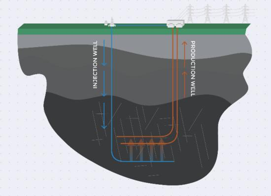
Horizontal drilling, which increases the contact area with the geothermal reservoir
