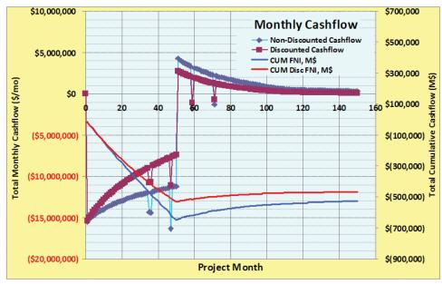
The Ryder Scott economic analysis shows negative cash flow for a typical Montney project in which two wells are drilled each month for 50 months. Median EURs of 3,554 MMcf of gas per well were used based on type-curve analysis of more than 1,000 wells. Gas spot prices of about \$2 per Mcf and condensate at \$83.12 a barrel were used. The breakeven point for cash flow is \$4.12 per Mcf of gas. Drilling-and-completion costs were assumed to be \$7.9 million a well.
